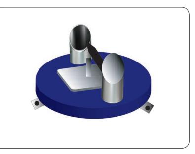
2. To adjust for too few tips (need less rainfall volume), raise the stop post on the opposite side of the bucket that is tipping too late. Re-lock the nut.
